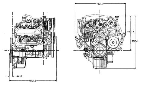
Figure 3.3.4.1 – L 4.3L V6 90 Degree Packaging Dimensions
